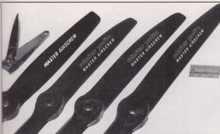
Curved leading edge of new Master Airscrew scimitar profile props lowers sound and seems to pull better. Fingernail clippers work great to lighten the heavy tip!
