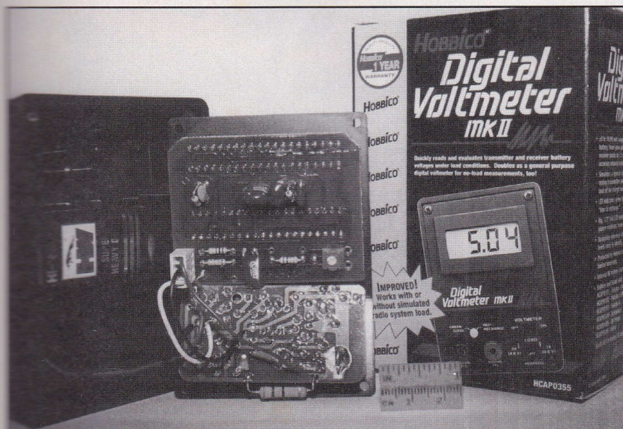
A single 9 volt battery (left, inside the black case) powers the new Hobbico Digital Voltmeter Mk II. Sophisticated internals ... works great.
